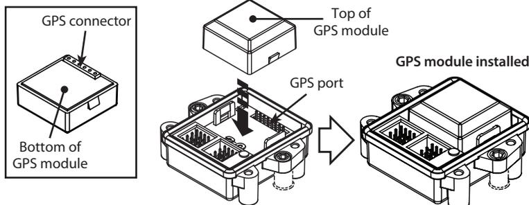
**Note:** Before reinstalling the expander cover, power up the system and verify that the GPS has linked, indicated by a solid green LED on the expander. If the LED is blinking red, there is an error in the system. Visit [Traxxas.com/telemetry](http://Traxxas.com/telemetry) for complete information and instructions on compatible devices and using the Traxxas Link App and the Telemetry Expander to capture and display real-time telemetry.
