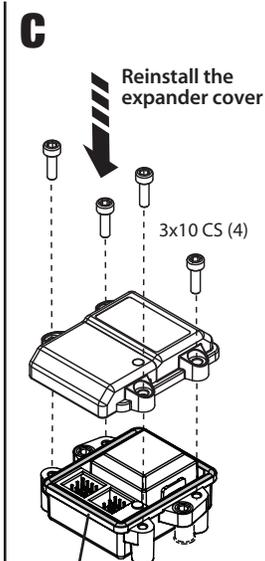
**Note:** Before sealing the cover on the Expander, ensure that the blue O-ring is properly seated in the groove.
